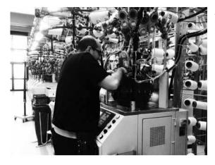
A knitting expert checking the workings of a circular-knit knitting machine.
